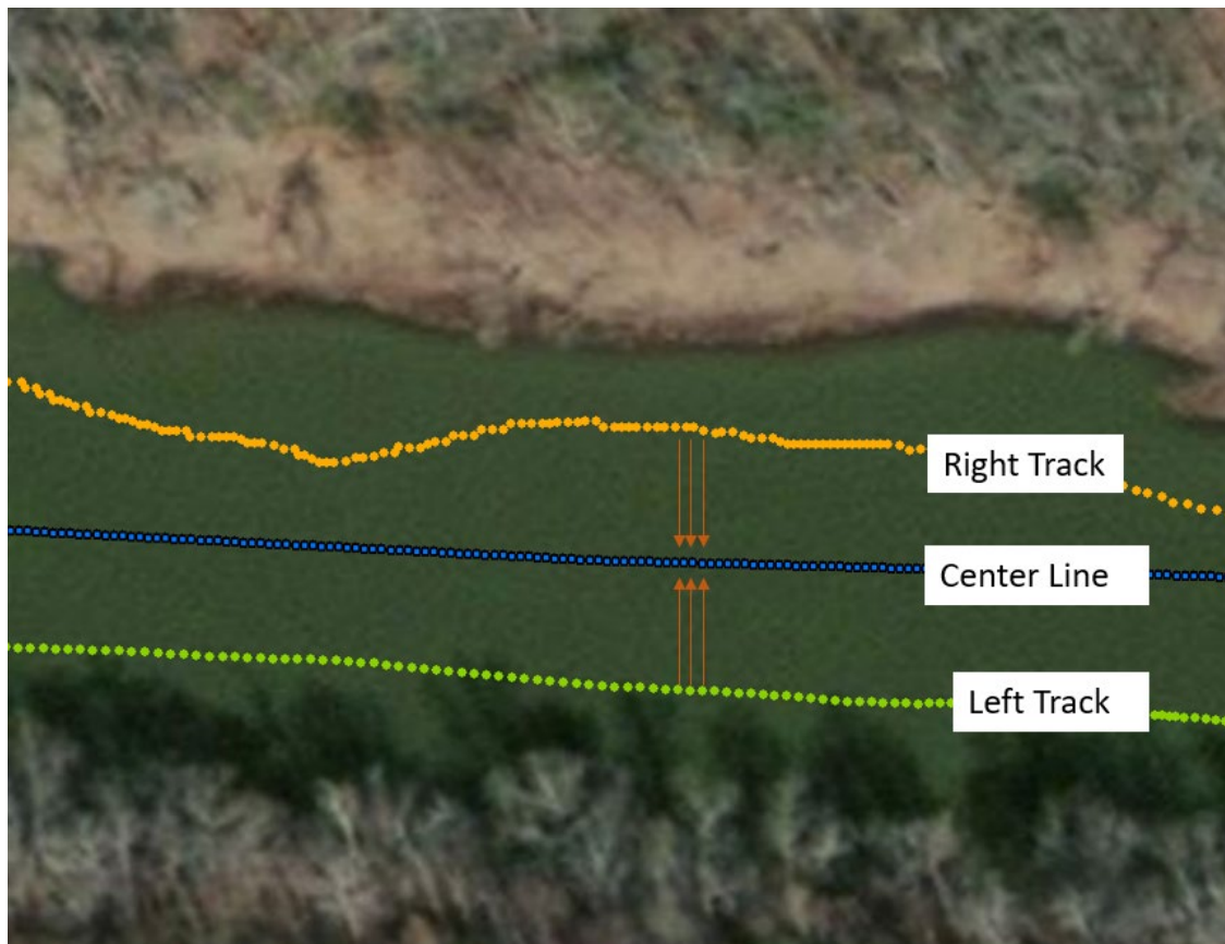
Figure 3: Example of mapping the data from the left and right boat survey tracks to a common centerline to allow the comparison of data at a single location.
