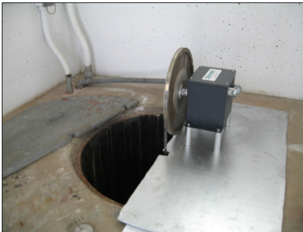
Figure 5-1. Typical Encoder with Wheel Tape for Measuring the River Stage or Lake Elevation in a Stilling Well
